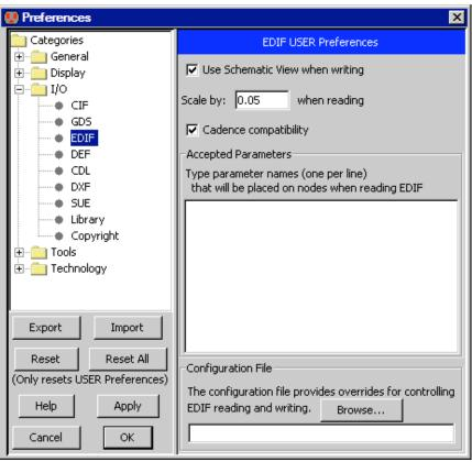
The bottom section of the panel lets you specify a configuration file that will control EDIF I/O. This file has conversions between coordinates and names inside of Electric and the EDIF file. The file has these lines of text that control different aspects of conversion:
