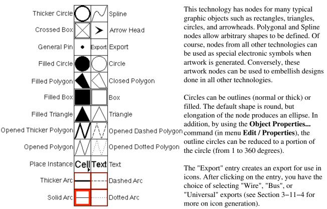
There are four different polygon styles: opened, closed, filled, and spline. The opened polygon can be drawn with solid lines, dotted lines, dashed lines, or thicker lines. These nodes require that you use the "Outline Edit" mode (see Section 6-10-1).
