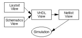
When simulation is requested, the cell in the current window is simulated. Date checking is performed to determine whether VHDL translation or netlist compilation is necessary. If you are currently editing a VHDL cell, it will not be regenerated from layout, even if the layout is more recent. Similarly, if you are currently editing a netlist cell, it will not be regenerated from VHDL, even if that VHDL is more recent. Thus, simulation of the currently edited cell is guaranteed.
