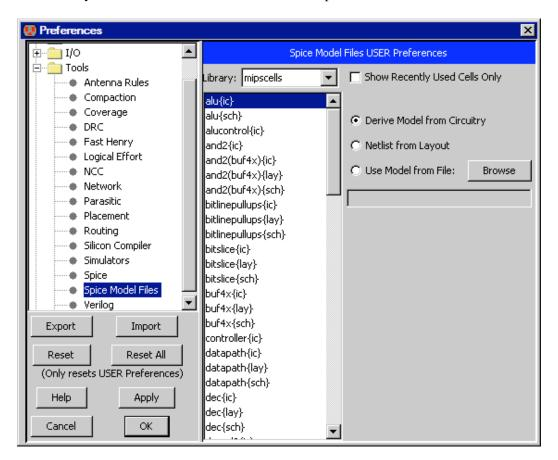
The same function can be done by using the **Set Netlist Cell From File** command (in menu **Tools / Simulation (Spice)**). This places a piece of text in the cell, which you must edit to be the path to a disk file. That file will then be included in the Spice deck instead of the actual subcircuit of the cell.
