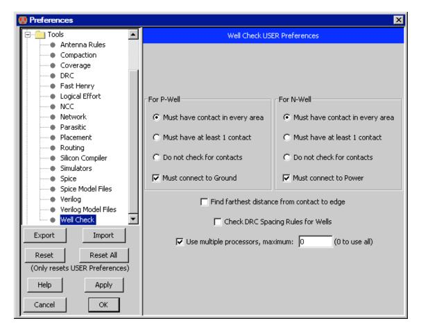
The Well Checker makes sure that there are well contacts in every area of well. The dialog allows you to relax that restriction and demand only 1 well contact in each cell, or not to check for contacts at all.
