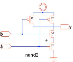
These symbols are *nodes* in Electric parlance. You may move the nodes around by clicking and dragging. The transistors default to a width/length value of 2/2. Double–click on the pMOS transistor and change its width to 12. Recall that nMOS transistors are roughly twice as strong as pMOS transistors. So a single nMOS transistor would only have to be 6 wide. However, because the nMOS transistors are in series, they should also be 12 wide.
