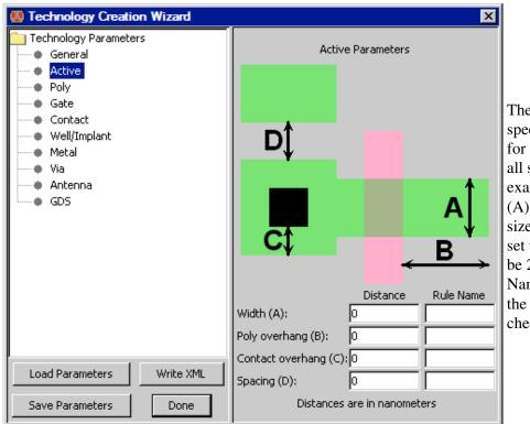
The "Active" panel lets you specify size and spacing values for the Active layer. Note that all sizes are in nanometers. For example, if the Active Width (A) is set to 200, and the Unit size (in the General panel) is set to 100, then Active arcs will be 2 units wide. The "Rule Name" fields let you describe the rule so that the design-rule checker can report error names.
