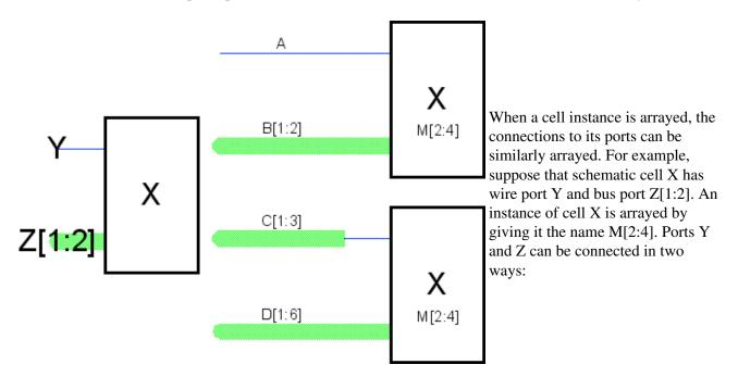
Implicit connection to all instances (top illustration). If the wire port Y is connected to a single wire (A), then wire A connects to port Y on all three instances of cell X. If the bus port Z is connected to a 2-wide bus (B), then each element of that bus connects to the same element of bus port Z on all three instances of cell X. So B[1] connects to port Z[1] and B[2] connects to Z[2] on all three instances, M[2], M[3], and M[4].
