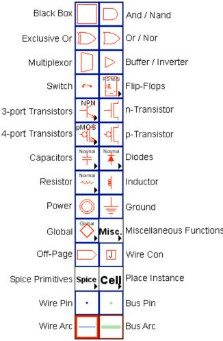
The Schematic technology allows you to design using digital and analog schematic components. To obtain this technology, use the popup menu at the top of the component menu and select "schematics".
