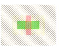
Although the default transistor is 2x3 in size, most people want them to be wider. For the purposes of this example, make the transistor be 12 wide. To do this, select the node and use the **Object Properties** command (in menu **Edit / Properties**).
