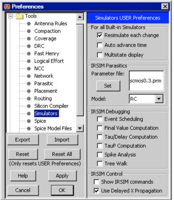
Advanced users who edit their own command files may enter specialized IRSIM debugging commands. These commands depend on a set of flags to determine the type of debugging to do. Checkboxes in the "IRSIM Debugging" section control these debugging flags.
