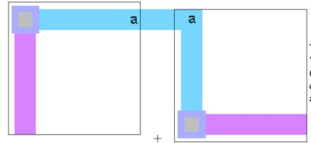
The top level of hierarchy (cell "high") has two instances of the cell (the right instance is rotated 90 degrees) and an arc connecting them, as shown here.
