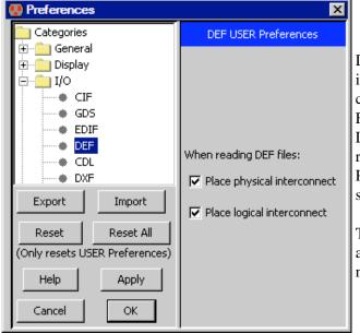
DEF (Design Exchange Format) is a recent interchange format for CAD systems. It is often combined with LEF (Library Exchange Format) files. For more information on reading and writing DEF or LEF, see Section 3–9–2 and Section 3–9–3, respectively. DEF options are controlled with the DEF Preferences (in menu **File / Preferences...**, "I/O" section, "DEF" tab).
