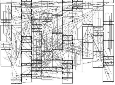
Another way to get Unrouted arcs for router input is to use the **Copy Routing Topology** and **Paste Routing Topology** commands. These copy the network topology from one cell (the "copied" cell) to another cell (the "pasted" cell). The copied cell should be properly routed. The **Paste Routing Topology** command uses node and arc names to associate the two cells.
