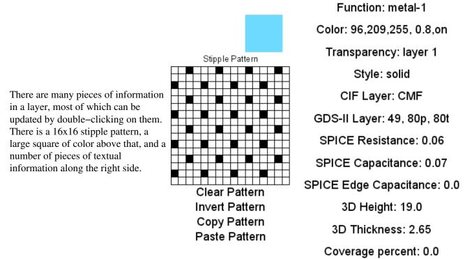
The stipple pattern can be changed by double–clicking on any grid squares. You can also do operations on the entire stipple pattern ("Clear Pattern", "Invert Pattern", "Copy Pattern", and "Paste Pattern") by double–clicking on their name below the pattern area.
