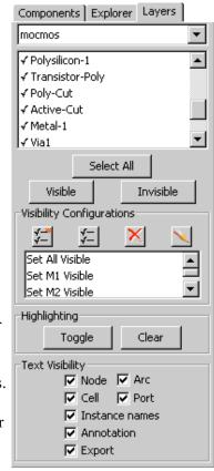
You can also customize these commands so that an arbitrary combination of layers is visible. To do this, set the desired layer visibility, click on an entry in the "Visibility Configurations" section, and click the "Save Visibility" icon (second from the left at the top of the "Visibility Configurations" section). To rename an entry, use the "Rename" icon (rightmost icon).
