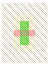
Start with a transistor (in this example on the left, an n-transistor). Rotate the transistor so that the gate is vertical. To do this, use the **90 Degree Counterclockwise** command (in menu **Edit / Rotate**), or just type Control–J. Note that the active gate on the left is highlighted (it is just a line).
