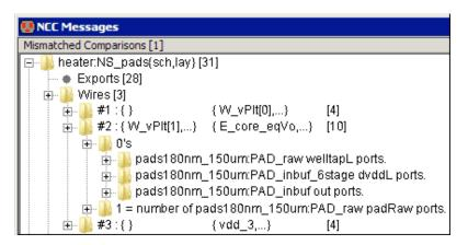
When a wire class node is selected, the right half of the window displays a two–column table (see figure below). Each column corresponds to one of the compared cells and has a list of that cell's wires which belong to the selected wire class. Matched wires are printed in green, the two wires on the same line match each other. Mismatched wires are printed in no particular order.
