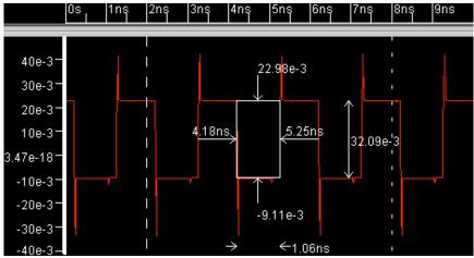
Another way to measure in the waveform window is to use the "measure" tool (see Section 4-7-4). This tool lets you drag a rectangle, and it shows the left/right time with difference as well as the top/bottom values with difference. The tool snaps to data points so it is easy to get precise measurements.
