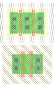
Once the contacts are connected to the transistors you will need a gap of only 1 unit between the metal and polysilicon. Use the design rule checker to ensure you are as close as possible but no closer. Using similar steps, draw two pMOS transistors in parallel and create contacts from the P–diffusion to Metal–1. At this point, your layout should look something like this.
