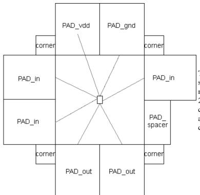
This file places 8 pads in a ring (2 on each side) and also places corner "pads" for making bends. The input pads connect to the 2 input ports "a1" and "a2". The output pads connect to the 3 output ports "out1", "out2", and "out3" The power and ground pads connect to the "vdd" and "gnd" ports.
