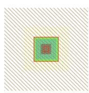
Next we need a contact. Choose a "Metal-1-N-Active-Con" to connect the N-Active to Metal-1. Make its size be 5x12 instead of the default 5x5. Notice that contacts are "smart" about the cuts, and add them to fill the node. Note also that the port (the inner rectangle) grows with the node.
