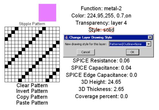
Because every layer has a default stipple pattern used for printing, all that is necessary is to change the "Style" field from solid to patterned. To do this, double–click on the "Style" text and select "Patterned/Outline=None". The technology is now modified and can be converted back with the **Convert Library to Technology...** command.
