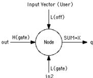
Driving inputs may be from other simulation nodes, in which case the driving strength is "gate" (i.e. H(gate) indicates a logic HIGH state with gate driving strength), from a power or ground supply ("VDD" strength) or from the user (any strength). If no user vector has been input at the current simulation time, then the input defaults to the "off" strength.
