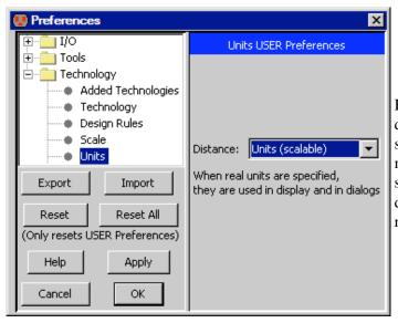
By default, distances are expressed in dimensionless units, and the true unit size is shown in the status bar. The Units Preferences (in menu **File / Preferences...**, "Technology" section, "Units" tab) allows you to request that dimensions be shown in real units, such as nanometers.
