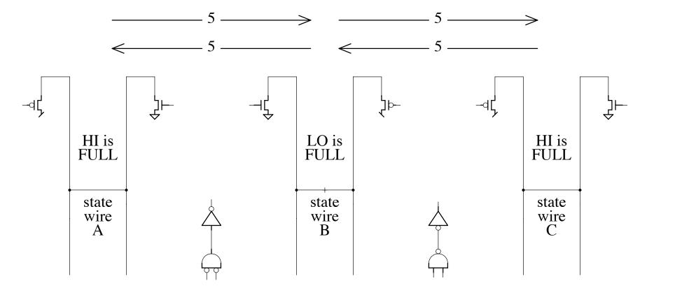
add wires, transistors and inverters to complete the two 5/5 stages
