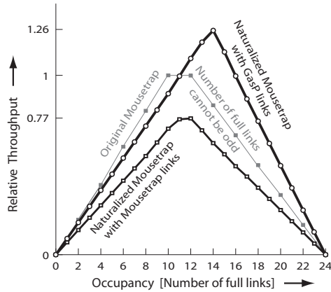
Figure 8 Three canopy graphs for simulations of rings with 24 pipeline stages. The center graph with fewer data points is from simulation with an original Mousetrapp module. Naturalizing its links with the circuit of Figure 6(c) produces the lower graph. The increased number of logic gates costs performance. Using the link circuits of Figure 6(b) produces the upper graph, improving the original performance. These three 90nm simulations omit data latches and wire loads.
