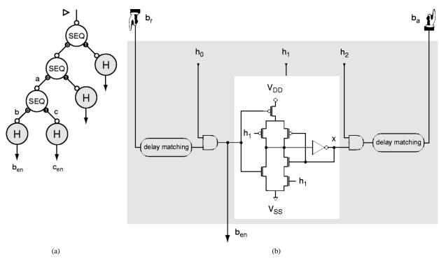
**Fig. 10.** New circuit configuration with (a) HOLD DfT and (b) a straightforward implementation for HOLD. The delay for the DfT circuitry is compensated in the delay-matchings for the data-path operation (see Fig. 7).
