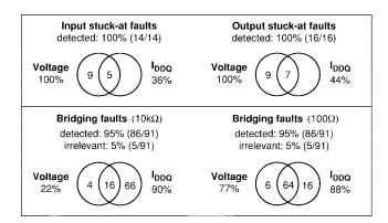
Fig. 11. Simulated fault coverage for SEQ with HOLD DfT.
