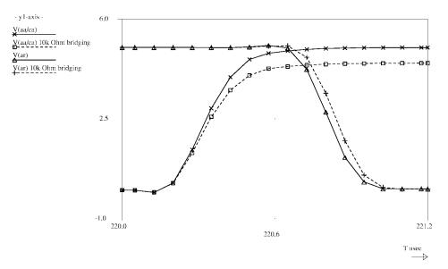
**Fig. 5.** Detail of the 10-k $\Omega$  bridging fault simulation in Fig. 4(b), showing the increased path delay from  $a_a$  rising to  $a_r$  falling compared to the fault-free situation. For high-resistive bridging faults, such as in this case, the changes in propagation delay typically are marginal, and the circuit will function correctly.
