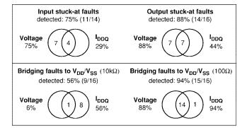
Fig. 9. Simulated fault coverage for control component SEQ.
