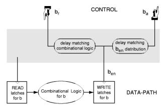
**Fig. 7.** Handshake interface between the control and a single-rail data path. A four-phase handshake over  $b_r$  and  $b_a$  generates a pulse on  $b_{en}$ , which makes it possible to capture the results from the combinational logic in the level-sensitive latches in a way similar to clocked data paths. A circuit can have many data paths that may share combinational logic and latches but typically have their own handshake control channel.
