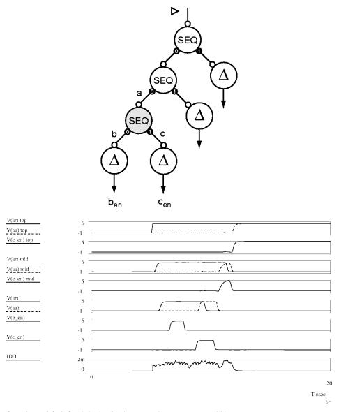
Fig. 6. Simulated configuration and fault-free behavior for three control components SEQ driving four data paths  $\Delta$  (see also Fig. 7). Faults are injected in the grey-colored SEQ component, and the fault effects are tested in the two initial and final quiescent states.
