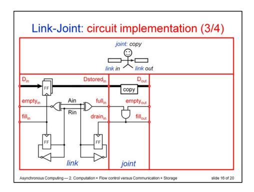
The joint can be implemented as a simple AND gate for ANDing a full in with an empty out.
