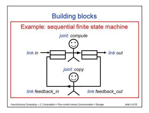
The computer scientists in the audience will appreciate that this link-joint model can create a sequential finite state machine <CLICK>
