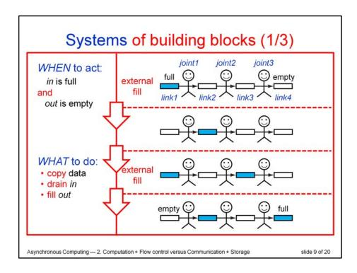
We can build a First In First Out buffer, or FIFO, by connecting multiple links and joints in series, as in this picture.
