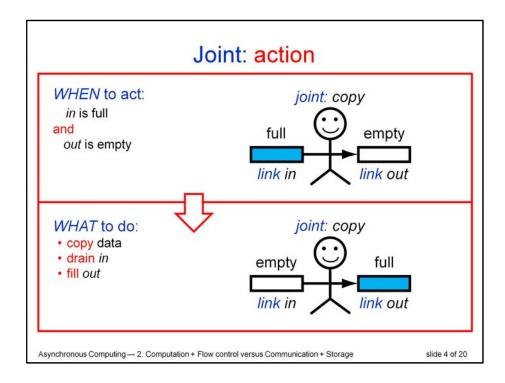
Here is an example of a simple joint that copies data from its input link *in* to its output link *out*. The joint can either do nothing or act.
