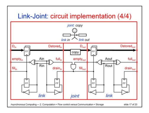
The output link can have the same implementation as the input link.
