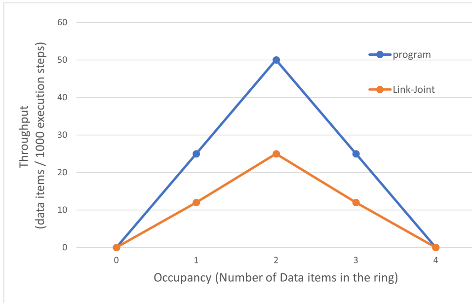
Figure 6.10: Canopy graph showing the simulated throughput of the ring FIFO with varying numbers of data items at different abstraction levels.
